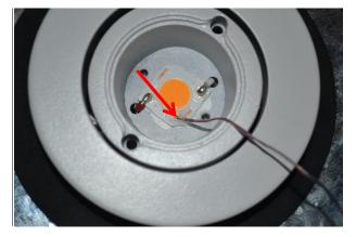
Temperature measurement point of driver (TMP<sub>c</sub>)
